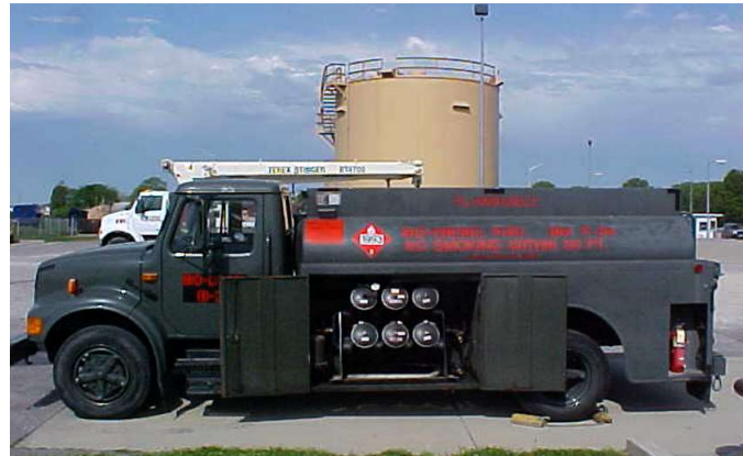
U.S Air Force installed Model 6175 (78 gpm max.)
